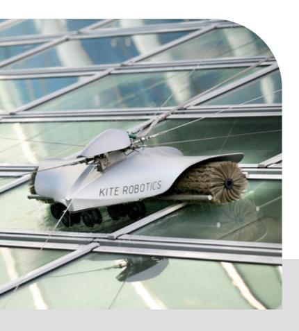
Having two versions of the model on the market, allows both vertical and horizontal façades to be accessed and cleaned.
